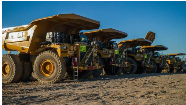
240-tonne rigid frame haul trucks
